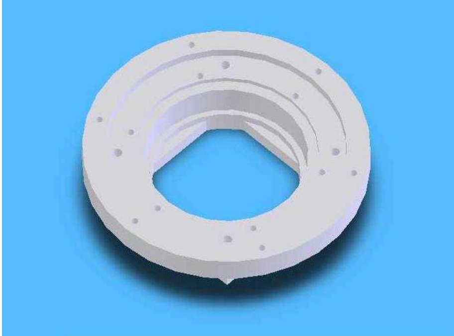
Figure 4.1: Drawing of attachment for Apogee CCD camera. We designed this attachment to house the CCD camera and fit against the Goodman Spectrograph temporarily.
