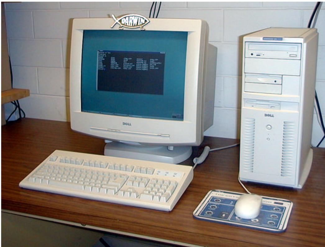
Figure 2.2: Darwin, the master computer controlling all 64 nodes.
