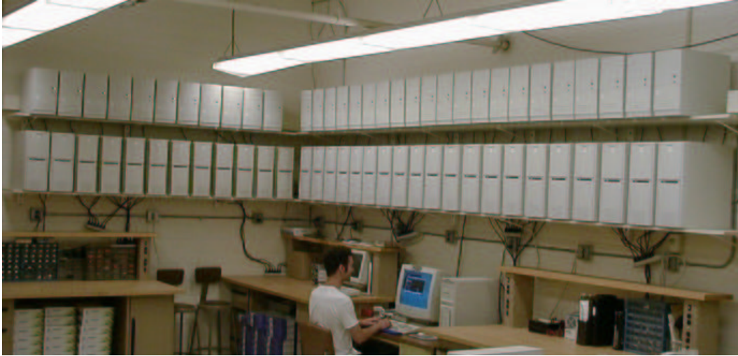
Figure 1.3: This metacomputer is a collection of 64 minimal PCs connected by a network, and can calculate our white dwarf models in parallel.
